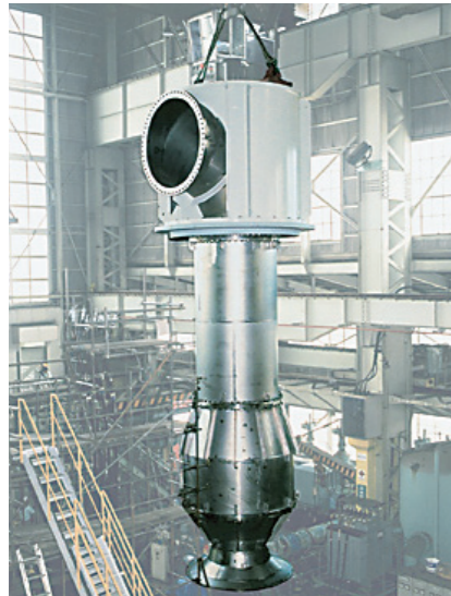
Seawater Pump (S31803, S32760, S32750)
